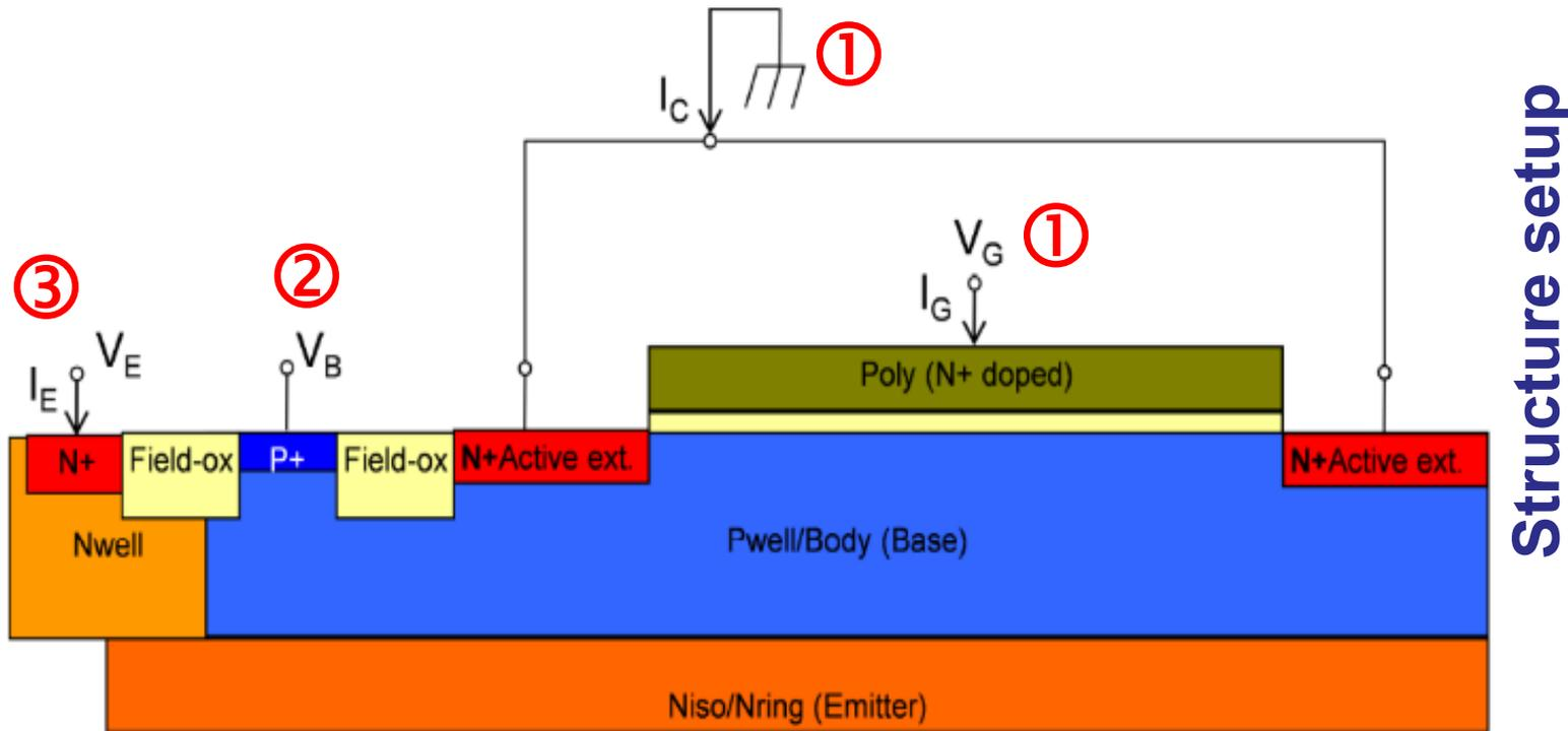
✓ Conventional nMOS with additional emitter region to control the hot-electron injection into the body
